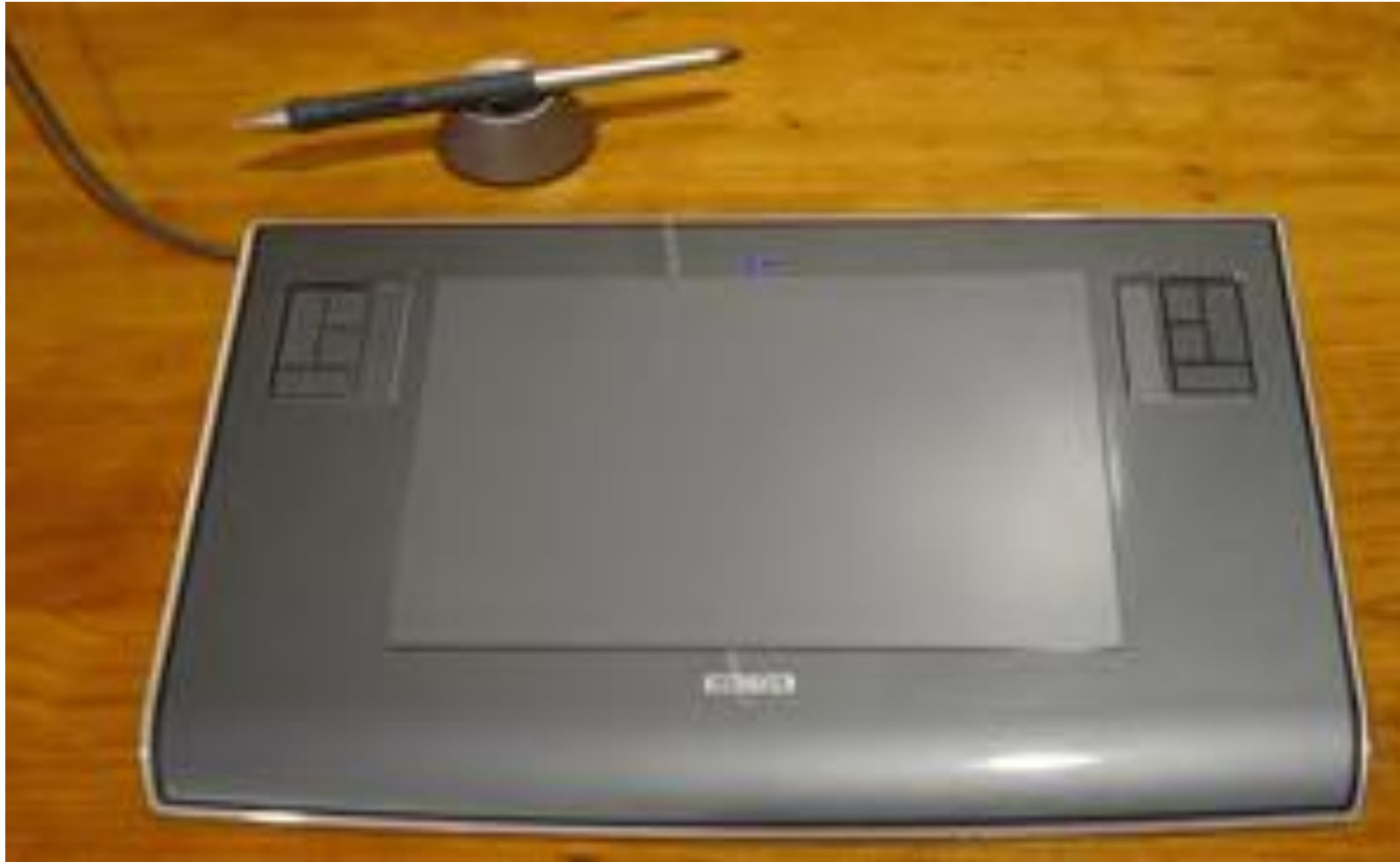
Figure: A tablet with a specially designed pen to write with is another application of magnetic induction.
