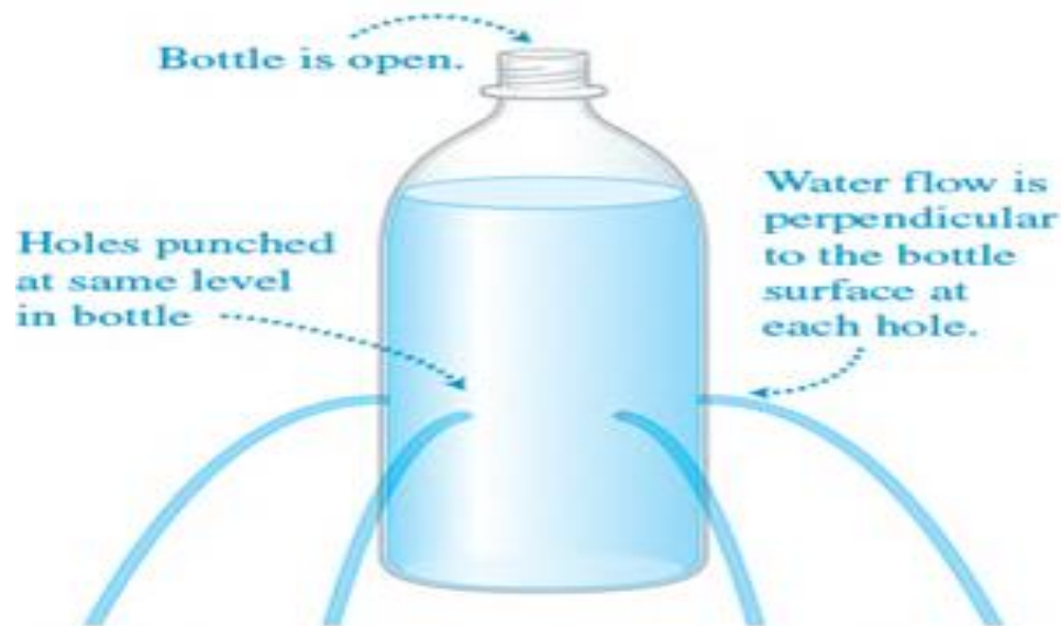
Figure Arcs of water leaving holes at the same level in a bottle.
